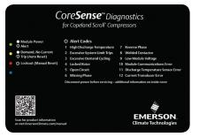
All large refrigeration Copeland Scroll compressors come equipped with CoreSense ™ Diagnostics.
