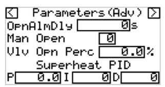
Open Alarm Delay - if Manual Open = FALSE and the valve stays open at maximum value for a time longer than Open Alarm Delay an alarm will occur. The alarm resets automatically if the output changes to a smaller value.
