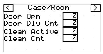
**Door Open:** displays when physical Digital input (*Door Switch*) is active. **Door Delay** is based on time set in setpoints for open and close for counting.
