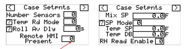
If using the M172DCL display HMI select 1. If no remote display is used, select 0 and reboot PLC!
