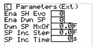
If **SH Evolution Enable** is set to "1", the superheat control is performed with an advanced algorithm, instead of the standard PID. *See Schneider's Manual (Modicon M172 Electronic Expansion Valve Driver)* for more information.
