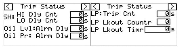
**SH(Superheat)** High and Low delay Count – Delay Count, that was set in Setpoints, before we trip an alarm. If SH High or Low value is reached, this time must expire before we alarm and wait for manual reset.
