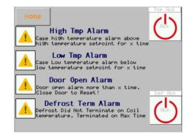
\*\*NOTE: NO ALARM ACKNOWLEDGE CAN BE MADE WHEN YOU ARE NOT READING FROM HMI SELECTED IN SETPOINTS!!
