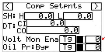
If toggled to select "1", system will look for Physical DI (*see wiring schematic*). If this input is not active, System will alarm and shut down.
