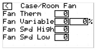
Evaporator Fan Thermal (If Present) – 1 = State is Ok to run. Digital Input is True. 0 = Trip or not present. Digital Input is False.
