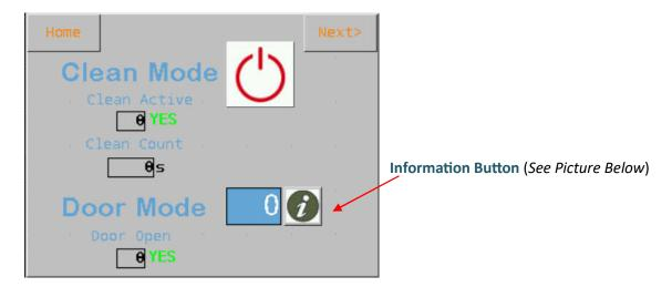
**Clean Mode Push Button** will illuminate green when pressed and red after 4 seconds of being released. This will force the system into **Clean Mode** and count to time set from PLC.
