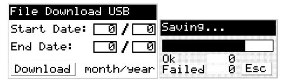
Select the **start** and **end date** at which you want to pull the above data to a USB. Set the same start and end date to pull data for that month. **OK** = **1** means the data was successfully transferred to the USB.
