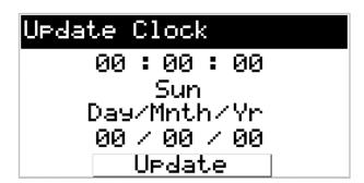
**Updating the RTC** is important when pulling data from the device. This will make it easy to trace a specific time and date at which an error has occurred in the system.
