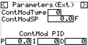
Continuous Modulation: Used to control case Temperature for Sensori M172-18IO Case Management
