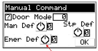
Door Mode – 0 = Auto mode. This mode is waiting for the physical Door switch (DI), to be active before the count will start. When a count has expired, based on setpoints set for Door open/Close delays, the system will shut off.
