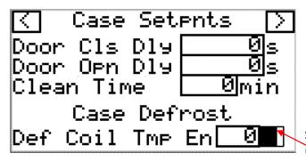
Set to 1 if a **Defrost Coil Temperature** is being
