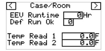
**EEV Runtime** – Status of Electronic valve runtime. Used to determine Defrost, when "Defrost Runtime" is enabled. Value MUST be "1" and "ok", for a defrost to run its cycle. See Below Setpoints for further details
