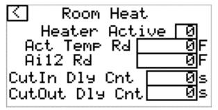
Heater Cut in and Out Delay counts in seconds.
