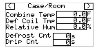
Combination Temperature - used to control refrigeration on/off (Control Temperature). Depending on Number sensors and "Temp Rd Md" selected in Setpoints. This will show the combined method of case/product temps. If only one temp active, "Temp Read 1" will display the same, and "Temp Read 2" will display 0.
