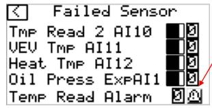
**Temp Read Alarm** Indicates failed sensor for "Tmp Reads" when selecting "Number of Sensors". Also, can indicate if "Temp Rd Mode" 4 is selected and number of sensors DOES NOT equal 2. When an Indication of "1" is present, a sensor alarm has been reached.
