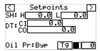
**Suction SH: High, Low** – Range 0-50F. **Superheat High** is the value at which you want to protect the compressor from overheating. Overheating the compressor occurs above 20F and RE and efficiency is lost. **Superheat Low** must be set to protect the compressor from flood back. AN INITIAL DELAY IF HIGH SUPERHEAT OR LOW SUPERHEAT, IS 60 SECONDS BEFORE IT LISTENS TO THE SETTABLE HIGH AND LOW SUPERHEAT DELAYS. **DEFAULT: HIGH=30F, LOW=0F**
