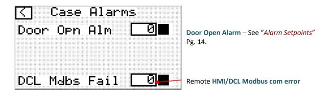
If Voltage Monitor is present and there is no active input made (*see wiring schematic*), then this alarm will be active.
