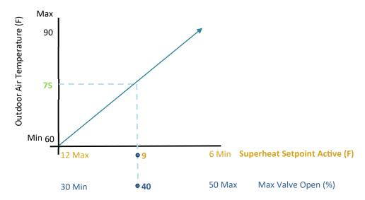
On This Graph, Superheat Shift Active setpoint would be 9-degree F and Max Valve Open Shift Setpoint would be at 40%, at a 75-degree F ambient day.
