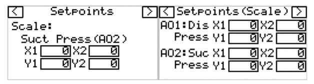
Scale - Scaling for Analog Output 1 and 2 for Discharge / Suction Pressure Out. 0-5vdc output only. Set "X" as Pressure scaling in REAL value. Set "Y" as voltage scaling in integer format (ex. 500 = 5vdc)
