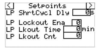
LP Short Cycle Delay- Delay at which the compressor will be off for, after the "cut in" value was reached. Set this value to avoid compressor start/stops on a low pressure alarm. Value set in seconds. **DEFAULT=180 seconds**
