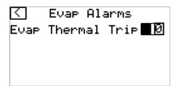
**Evaporator Thermal Trip** – value of "1" when an evaporator thermal motor trip has occurred, enabled in setpoints. If Evaporator thermal is enabled in setpoints and the digital input (See wiring schematic) is true, then no alarm will be present. When this input is false, a thermal trip will occur and only reset when the input is true again.
