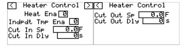
**Heat Enable** – Enables heater control for Room/Case.
