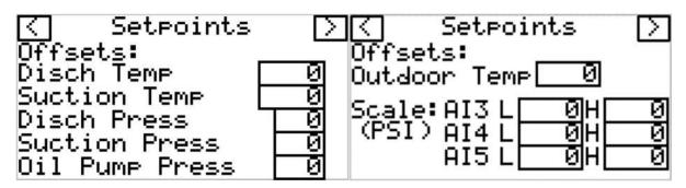
Offsets - Discharge Temperature, Suction Temperature, Discharge Pressure, Suction Pressure, Oil Pump Pressure, Outdoor Temperature.
