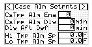
Case Temp Alarm Enable – Set to 1 if monitoring temperature for alarm state using the High and Low Temp alarm setpoints.
