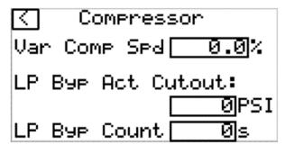
**Var Comp Spd** – Variable Compressor Speed Output from 0-100% being controlled through 0-10vdc Analog Output. See **Setpoints** for further information.
