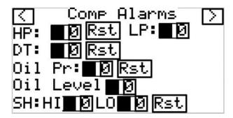
All Manual Resets located on first screen. High Pressure, Discharge Temperature, Oil Pressure, Superheat High and Low. These resets indicate beside "toggle" an indication of a trip status using the true value of 1. 0 indicates no alarm present. The toggle will also be highlighted black in a state of alarm.
