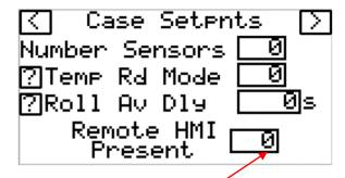
If using the M172DCL display HMI select 1. If no remote display is used, select 0 and reboot PLC! THIS IS SET IN AN INITIALIZE TASK AND SYSTEM MUST HAVE POWER RESET IF SET TO 0.
