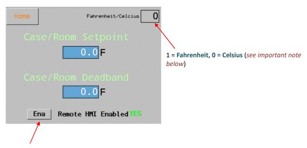
Once Enabled, this may only be removed by cycling power or taking control by the PLC! If Remote HMI and Sensori Case Management have two different power sources and power is cycled on either unit, The Remote HMI Enabled always defaults to the Sensori Case Management PLC.
