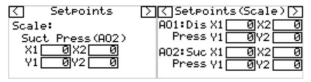
Scale - Scaling for Analog Output 1 and 2 for Discharge / Suction Pressure Out. 0-5vdc output only. Set "X" as Pressure scaling in REAL value. Set "Y" as voltage scaling in integer format (ex. 500 = 5vdc)
