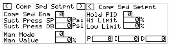
Compressor Speed Enable – Set to "1" to activate 0-100% variable speed control.
