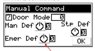
**Door Mode** – 0 = Auto mode. This mode is waiting for the physical Door switch (DI), to be active before the count will start. When a count has expired, based on setpoints set for Door open/Close delays, the system will shut off.
