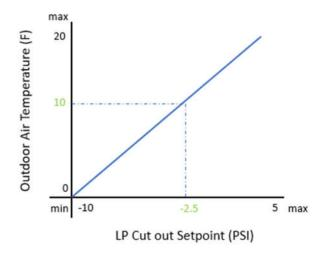
At an ambient temperature of 10 F, the new LP cut out will be -2.5 PSI for x time.
