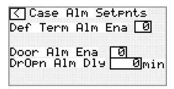
**Defrost Termination Alarm Ena** – Set to 1 if alarm is being used. If a coil temperature is present and maximum time is reached/do not terminate based on Coil temperature setpoint, in defrost, this alarm will be active.
