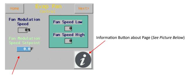
Fan Modulation Speed Setpoint can only be set/selected, when "Remote HMI Enabled" (YES)
