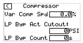
**Var Comp Spd** – Variable Compressor Speed Output from 0-100% being controlled through 0-10vdc Analog Output. See **Setpoints** for further information.
