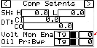
If Toggled to select "1", system will look for Physical DI (see wiring schematic). If this input is not active, System will alarm and shut down.
