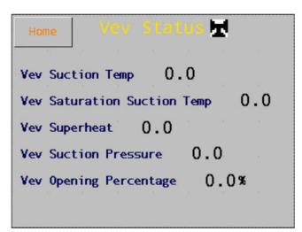
Vev Status Screen will not change from Celsius or Fahrenheit based on using the HMI degree change. This will always show the same status as what the Sensori Case Management PLC is Showing from the VEV parameter, dL08.
