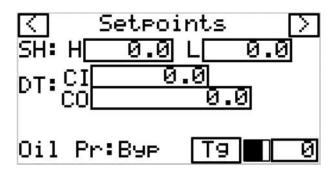
**Suction SH: High, Low** – Range 0-50F. **Superheat High** is the value at which you want to protect the compressor from overheating. Overheating the compressor occurs above 20F and RE and efficiency is lost. **Superheat Low** must be set to protect the compressor from flood back. AN INITIAL DELAY IF HIGH SUPERHEAT OR LOW SUPERHEAT, IS 60 SECONDS BEFORE IT LISTENS TO THE SETTABLE HIGH AND LOW SUPERHEAT DELAYS. **DEFAULT: HIGH=30F, LOW=0F**
