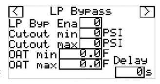
temperature min and max set. Set your "Cut out min" and "Cut out max" as a linear scaling reference setpoint. Set the "Delay" in seconds for how long the cut out value will be present for during initial start up. See below graph for example. Default Values: LP Byp Ena=0, Cutout min=-10PSI, cutout max= 5PSI, OAT min=0F, OAT max=20F, Delay=60 seconds
