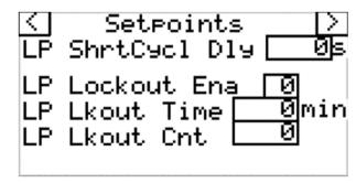
LP Short Cycle Delay- Delay at which the compressor will be off for, after the "cut in" value was reached. Set this value to avoid compressor start/stops on a low pressure alarm. Value set in seconds. **DEFAULT=180 seconds**
