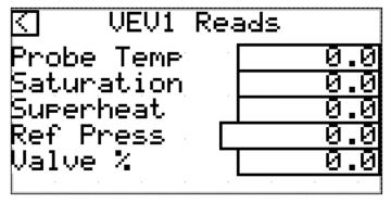
**Probe temp** – Temperature probe located on suction line at outlet of evaporator as installed by contractor.
