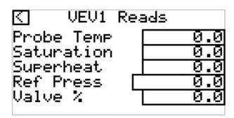
**Probe temp** – Temperature probe located on suction line at outlet of evaporator as installed by contractor.
