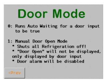
Door Mode – "Door Open" only displays from the physical DI door switch that is wired to PLC. This will not say that it is open if manual Door Mode is selected.
