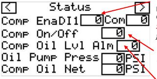
**Communication Enable**, used over Modbus protocol RS-485. This is only used when a Compressor Management Device is present. *See Sensori Compressor Management (section 1) for further details*.
