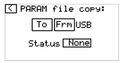
Parameter USB Backup and Restore- Insert USB and select "To" to backup all Eeprom parameters/Setpoints in Sensori PLC. Recommended to leave copy on site with PLC in case of future problems. To Restore Setpoints into a new PLC, simply insert USB with backup file and select "Frm" Usb to input USB eeprom files.
