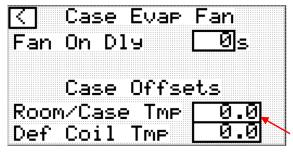
Fan On Delay – When Evaporator Fan is initially activated, it will delay for set time. Set this value low when using EXV to avoid valve from closing fully. If set too long on the M172-42IO, system could trip on low pressure. (0-45 SECONDS MAX)
