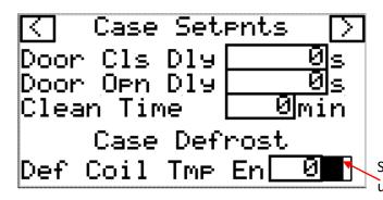
Set to 1 if a **Defrost Coil Temperature** is being used
