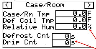
**Relative Humidity** only if present, 0 if not. Count Delays until **Defrost/Drip** expires based on time set in Setpoints menu.
