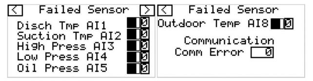
Displays/Indicates a **Failed Sensor** and which analog input it is. If oil pressure is not present and no sensor is installed, the value will remain to **0**, and no alarm will be present. If Low Pressure Bypass function is not used, this value will also remain **0** with no sensor installed.
