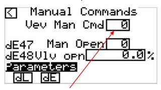
Like the previous screen – however, this is the internal command sent from the device to tell the valve to go into manual mode. Parameters **dE47** and **dE48** can only be used when there is a call for cooling/ the valve is active. When the valve is not active (*case is satisfied on temp, in defrost, or not enabled*), "Vev Man Cmd" may be used to force the valve using those selected parameters.
