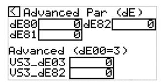
**dE80-dE82** parameters MUST be set to manufacturer specifications and max values. Damage to Valve can occur if settings are not correct! These changes can only be made when **dE00** = 0 (customizable)
