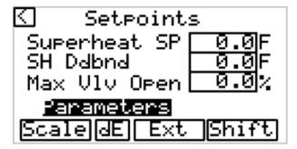
Set Superheat Setpoint for Electronic valve to modulate at.
