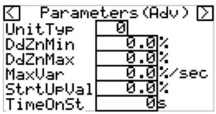
Unit Type - Type of unit to be controlled. If Unit Type = 0, parameters Superheat PID, Enable SH Evo, Superheat Deadband/DeadZone, MOP PID, Enable Dyn SP, Dyn Sp MxOf, SP Inc Step, SP Inc Time, are used as input for regulation.
